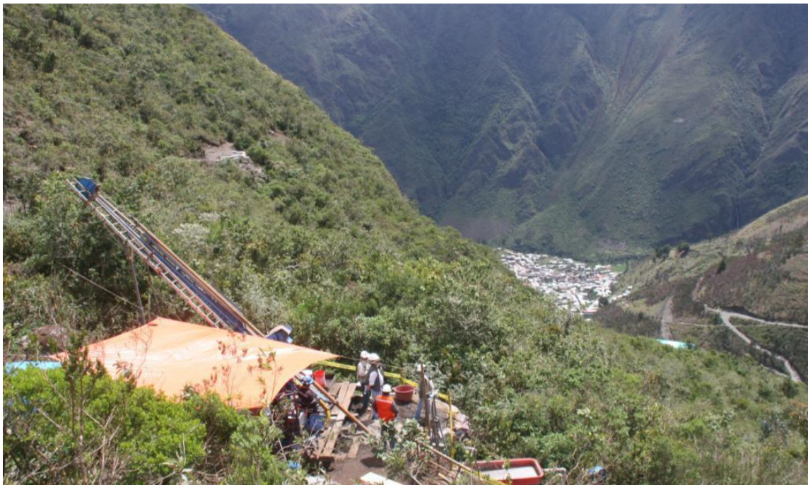
Figure 20 Diamond drilling at Minapampa East with Ollachea township in valley below
